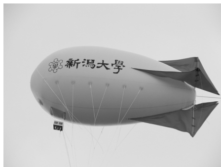
(a) Balloons used for establishing an ad hoc network in emergency situations
